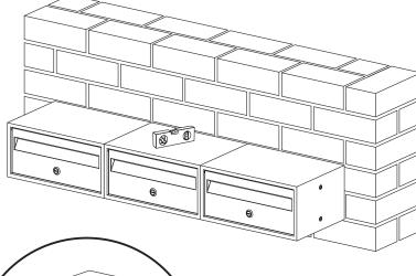
Open the front doors of all the letterboxes and mark the wall through the rear mounting holes.
