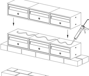
Once all letterboxes are in place, complete the remaining brickwork around the letterbox configuration.
