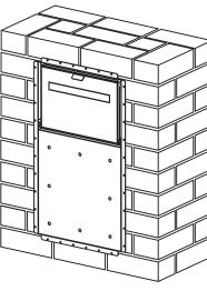
Once the brickwork and any rendering has been completed, attach the front panel by inserting the 8 x mounting studs through the corresponding holes in the back box. Reach through the back door and secure with the nuts provided.
