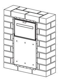
Once the brickwork and any rendering has been completed, attach the front panel by inserting the 6 x mounting studs through the corresponding holes in the back box. Reach through the back door and secure with the nuts provided.
